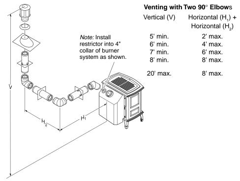
Figure 35 - Vertical Rigid Venting Configuration Using Two 90° Elbows with Two Horizontal Runs
